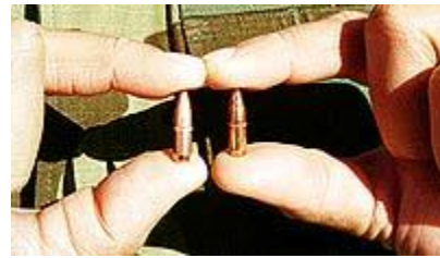
Figure 5: The tungsten-core 5.56 mm round on the left performs the same as the lead-core round on the right.
