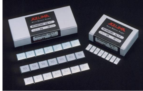
Figure 10: A selection of the steel adhesive weights produced by Azuma.
